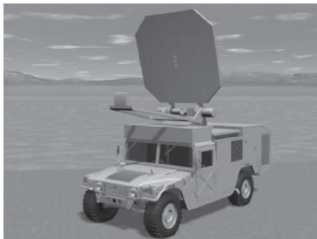
Figure 1. Artist's concept of mobile Active Denial System (ADS) to beam high power mm-waves (95 GHz).
